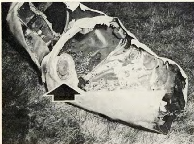
Damage in left tip tank cap area.
